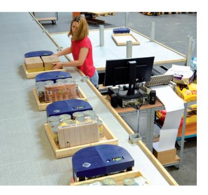
This was also the case with Futterplatz.de: construction and initial commissioning ran parallel to the previous operation; there was no classic standstill and relocation! Similar to a soft opening, the new storage system is continuously filled with goods and equipped piece by piece with more robots that move the goods carriers.
